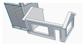
Now glue the walls together, the door walls fix to the inside of the gables as shown left.
